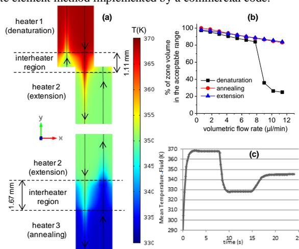
**Figure 2.** a) Temperature at a cross section (middle of the microfluidic channel height) of the unit cell of a fixed loop  $\mu$ PCR. The focus is on the interheaters region. Arrows show the direction of flow. b) The percentage of the volume of each zone in the acceptable temperature range (set point  $\pm 1.5$  K) vs. flow rate. c) The mean temperature of fluid during one thermal cycle in a stationary  $\mu$ PCR.
