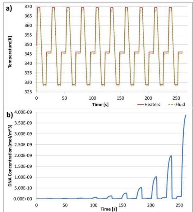
**Fig. 5** a) Temperature of the fluid and at the heater vs. time and b) DNA concentration in the static chamber μPCR device.
