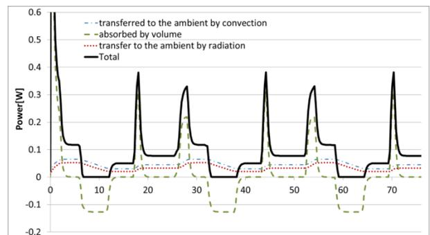
**Fig. 6** Total power, power absorbed by the volume of the unit cell, power transferred to the ambient by convection and radiation in the static chamber μPCR device for 3 PCR cycles. The total power needed at t=0 is 1.94 W.
