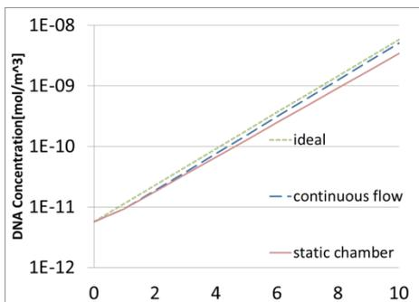
**Fig. 7** DNA concentration at the end of each thermal cycle for the continuous flow and the static chamber device; the ideal case, i.e. the case where the DNA concentration multiplies with 2 in every cycle is also shown.
