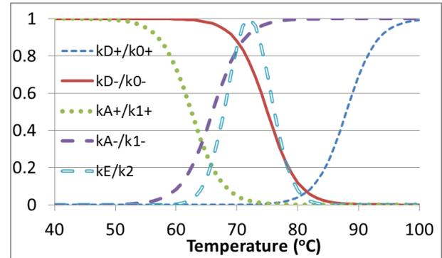
**Fig. 3** Normalized reaction rate constants vs. the fluid temperature
