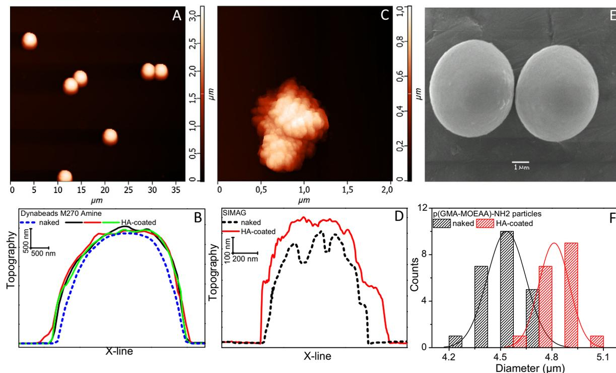
Fig. 2. Topographical AFM image of naked microparticles of Dynabeads M270 Amine and SiMAG (panels A and C) and corresponding illustration of the typical topographical profile of naked (dotted curve) and corresponding HA-coated particles (full-line curves – panels B and D). SEM image and histogram of the diameter of the naked and HA-coated p(GMA-MOEA)-NH<sub>2</sub> magnetic particles (E, F).
