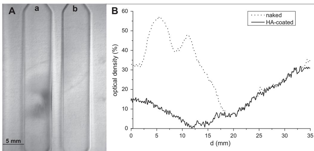
**Fig. 6.** A) The microfluidic channel of a PMMA microfluidic device after removing a) naked p(GMA)-MOEAA-NH<sub>2</sub>, and b) HA-coated p(GMA)-MOEAA-NH<sub>2</sub> magnetic particles (oligo-HA4); and B) plot lanes of densitometric analysis.
