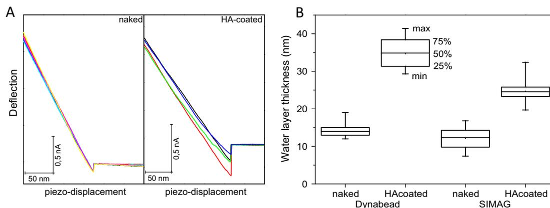
**Fig. 3.** AFM force spectroscopy of naked/HA-coated Dynabeads M-270 Amine particles illustrating an increase in the water thickness of the coated particles and the homogeneity of the HA-coating both on the Dynabeads M-270 Amine and SiMAG particles. See text for details.
