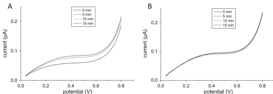
**Fig. 5.** Linear sweep voltammetry (LSV) voltammograms of hydrogen peroxide over time after contact with p(GMA-MOEAA)-NH<sub>2</sub>; A) naked particles, and B) oligo-HA4-coated particles: LSV, 1 mg L<sup>-1</sup> H<sub>2</sub>O<sub>2</sub> in phosphate buffer (0.1 M, pH 7.3) with 0.15 M NaCl, BST sensor Pt-Pt-Ag/AgCl; potential range 0–0.8 V, scan rate 0.1 V s<sup>-1</sup>.
