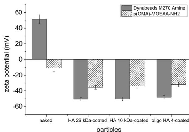
Fig. 1. Zeta potential of naked/HA-coated Dynabeads M-270 Amine and p(GMA)-MOEAA- $\text{NH}_2$  magnetic particles, coated by hyaluronic acid (HA) with varying molecular weight.
